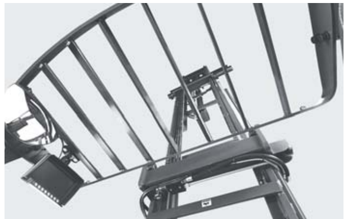
Optimised view through overhead guard
